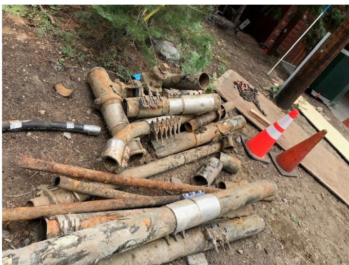
Above: Undersized and failing water pipes from the Tahoe Cedars Water System.
